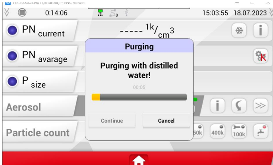
Figure 10: Progress display of flushing process
