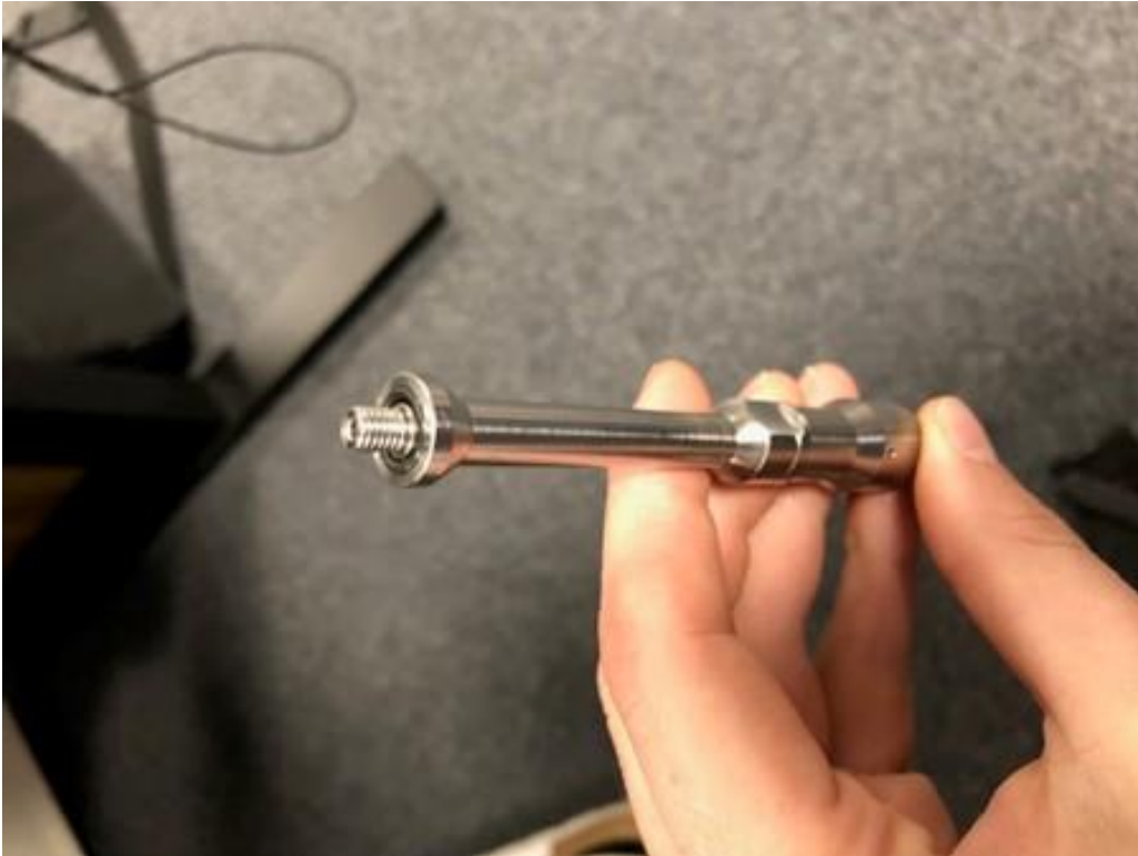
Figure 26: Nozzle (upper and lower part) of the salt generator
