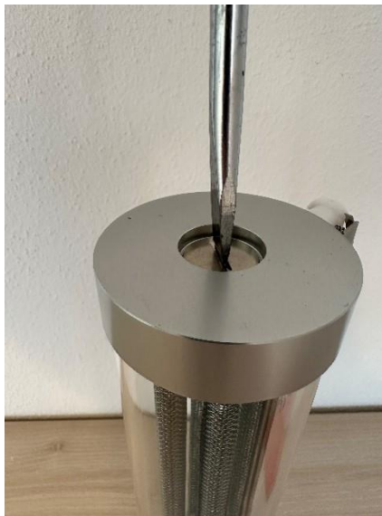
Figure 22: Open dryer cartridge (use screwdriver or coin)
